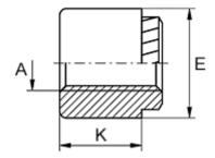
Female thread A = M5 Height K = 4 Hole diameter +0.1 = 6.8 Min distance to edge = 4.1 Min material thickness = 1.5 Outer diameter E = 9
